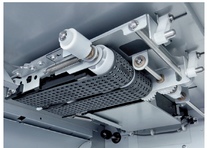
Incorporated vacuum feed technology for both paper feed units
