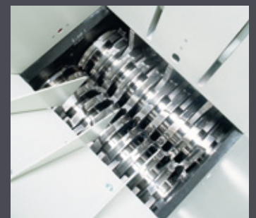
Cutting unit stage 1: Pre-shredder
