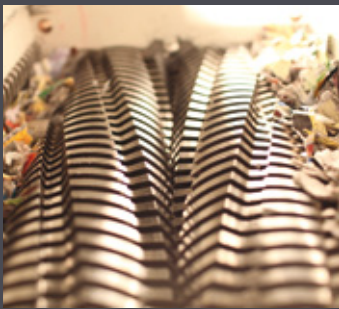
Cutting unit stage 2: downstream shredder
